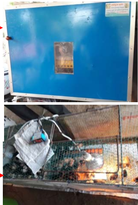
New machine from MB for hatching chickens with automatic temperature gauge (if temperature fluctuates, it adjusts automatically so farmer does not need to monitor all the time)
